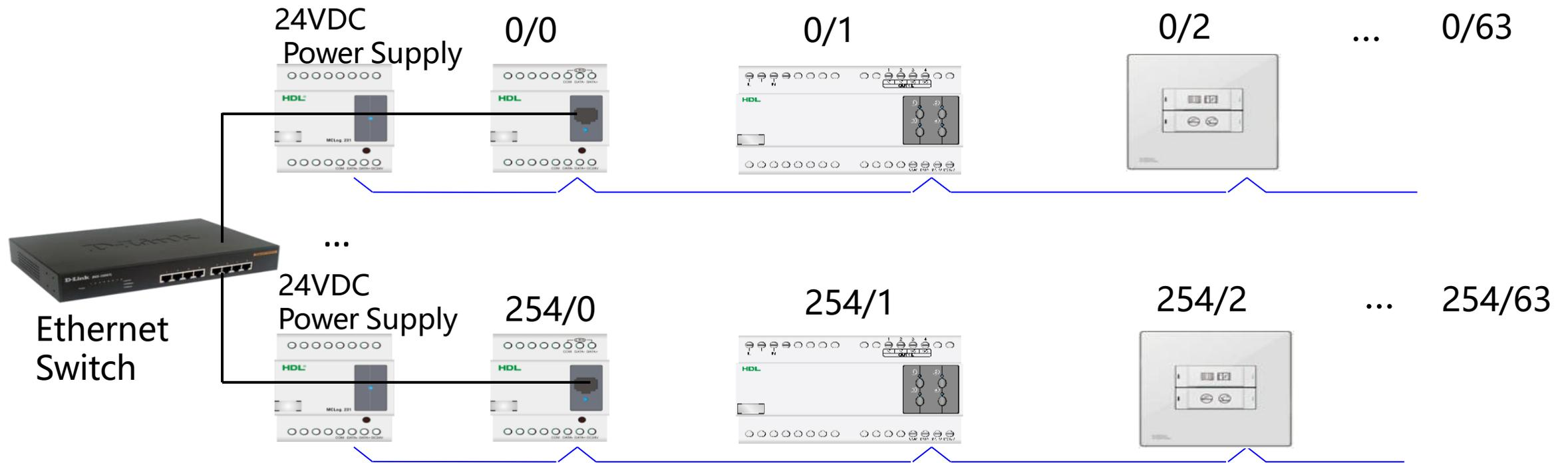
Every device has Subnet ID and Device ID except the Power Supply module, e.g., 1/2 means the Subnet ID = 1, Device ID = 2, the combination makes each device unique in the whole network.
