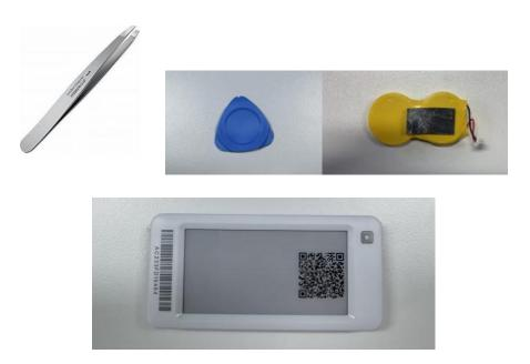
1. Find the disassembly port in the lower right corner of the ESL back cover, insert one end of the plastic triangle pry opening tool, move it around the gap between the back cover and the front cover. Remove the back cover of the ESL
