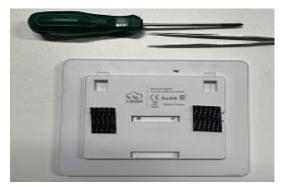
2. Find the disassembly opening in the lower right corner of the label, use a disassembly tool to pry open a small opening, and make a circle along the gap of the casing frame, and open the back cover of the label.
