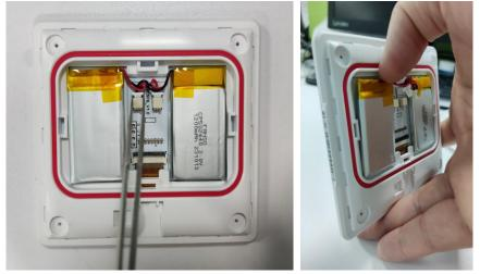
4. Install the new batteries (silk-screen one up, one down) with tweezers. Secure the battery with new double-sided tape and press the end of the battery for 3 to 5 seconds. Place the wire so that it does not rest on the fasteners and waterproof line.
