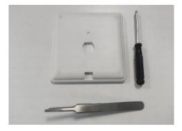
1. Remove the screw plug with tweezers. Remove the screws with a screwdriver.
