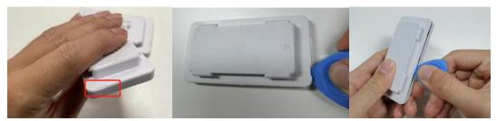
2. Place the label on the desktop with the screen down. Use tweezers to push out the battery connection terminals. If the battery connector of ESL is glued, cleaned off the glue.
