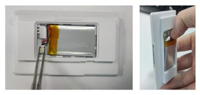
3. Install the new battery with tweezers (silk-screen down). Secure the battery with new double-sided tape and press the end of the battery for 3 to 5 seconds. Reinstall the battery cover.
