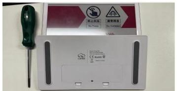
2. Open the back cover and replace 4 AA alkaline batteries.
