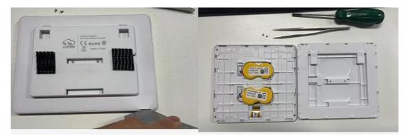
3. The battery connector interface of the factory product is glued, clean up the glue, and use tweezers to gently push out the battery cable. The new battery pack is pasted, fixed in the original position, and inserted into the battery connector. Install the back cover, press the frame buckle, and the replacement is complete.
