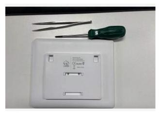
2. There is a disassembly opening on the left side of the rear case. Use a disassembly tool to pry open a small opening, and make a circle along the gap of the frame of the case, open the label back case, and take out the batteries one by one.
