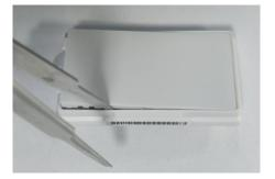
3. Remove the battery plug with tweezers. Pick the battery with your thumb (note: there are 2 pieces of double-sided tape fixed at the end of the battery)
